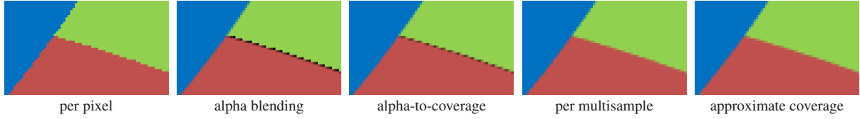
Figure 1: Example of curve rendering with 8 multisamples. While alpha blending and alpha-to-coverage fail at some interface pixels, both per-multisample evaluation and our approximate coverage technique yield good visual results.
