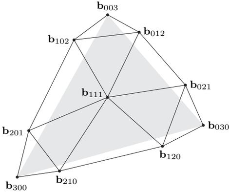
Figure 1: Control points  $\mathbf{b}_{ijk}$  of a PN triangle's cubic Bézier patch.
