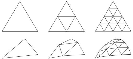
Figure 2: Refinement patterns for subdivision levels 0, 1 and 3 (top, from left to right) and their usage for tessellating a PN triangle (bottom).
