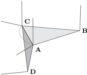
Figure 4: Adjacent triangles with different per-vertex normals at the common edge AC.
