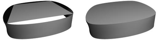
Figure 5: Holes in models (left) caused by specifying different normals for a vertex shared by multiple faces can be closed with connecting strips (right).
